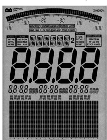
High-resolution digital pixel display (80x60mm) in FSTN quality with various numeric indicators, large bargraph and text display for simultaneous display of several measurement results and physical units.
